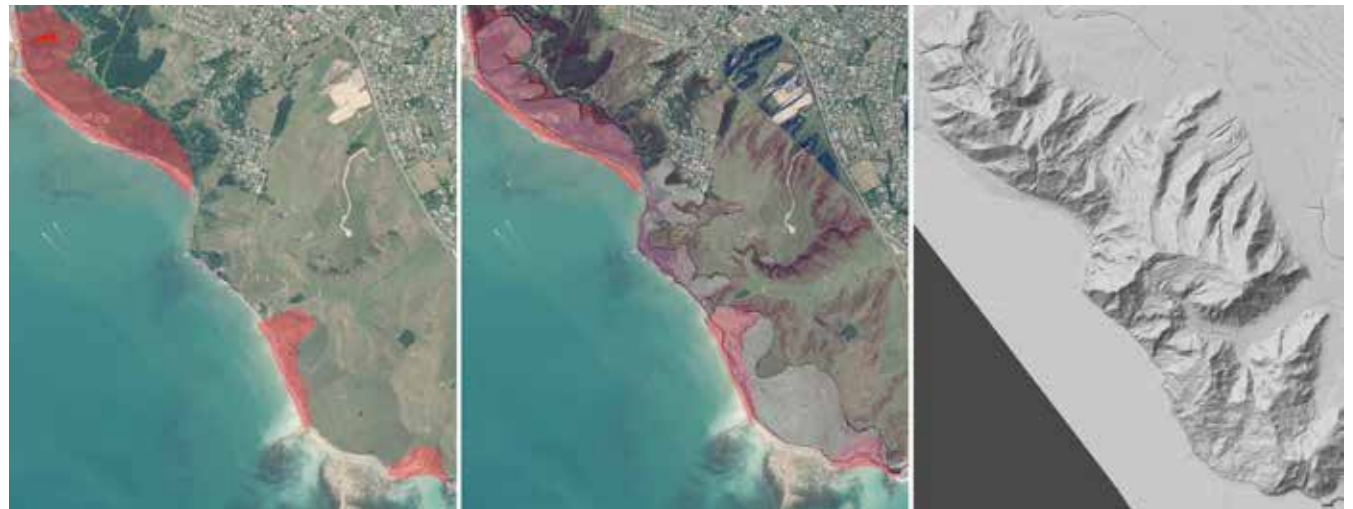
The 1st frame shows areas, in red, that are susceptible to flooding. The 2nd frame shows a more accurate representation of the areas that are susceptible to flooding. The 3rd frame shows the raw high-res 3D topographical data.
