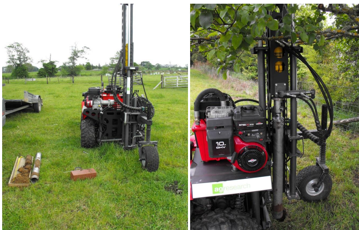
Figure 1. Hammer system in tower mounted on the rear of a modified quad bike for inserting soil cores. Core shown is 1050 mm length, 100 mm internal diameter.
