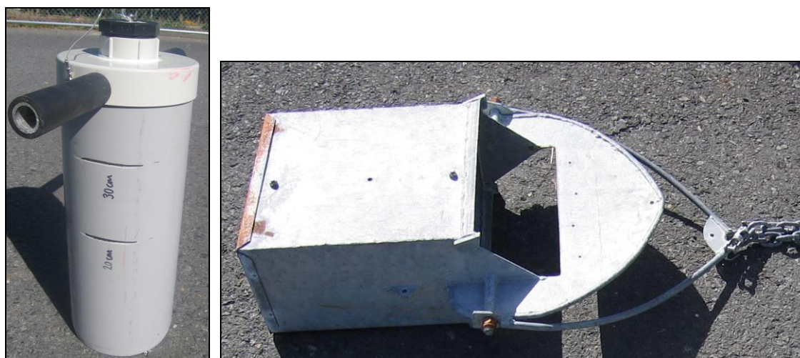
Figure 4: Large hand corer (left) and anchor box dredge (right) for sampling
