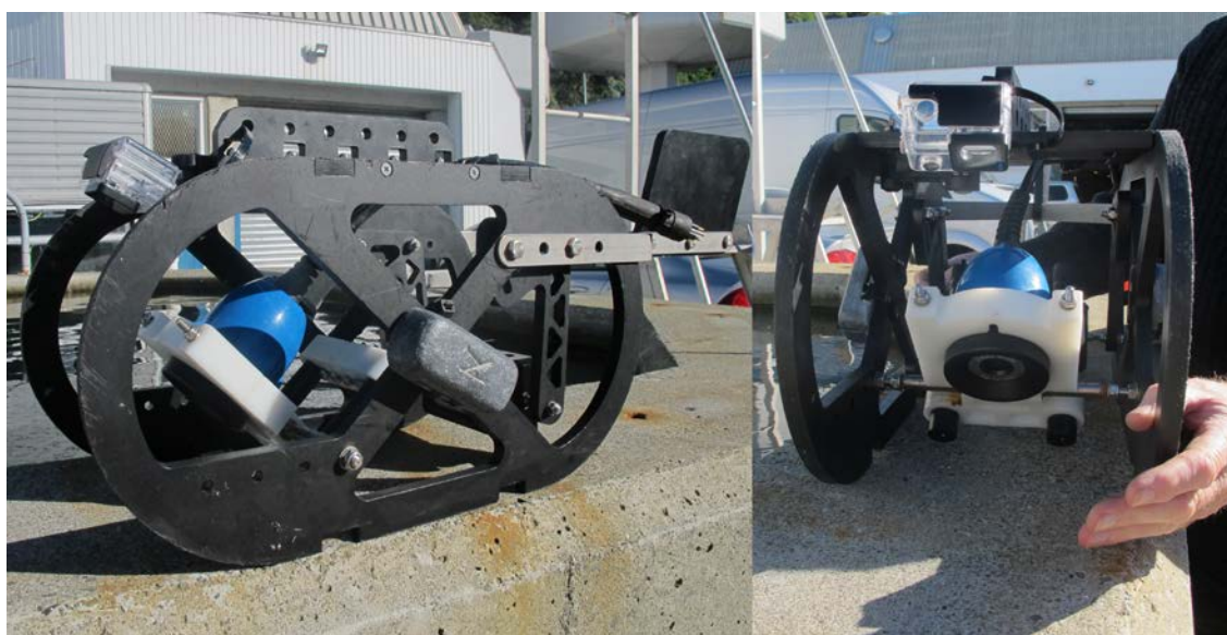
Figure 42: Towed camera system incorporating a splash cam and a GoPro.
