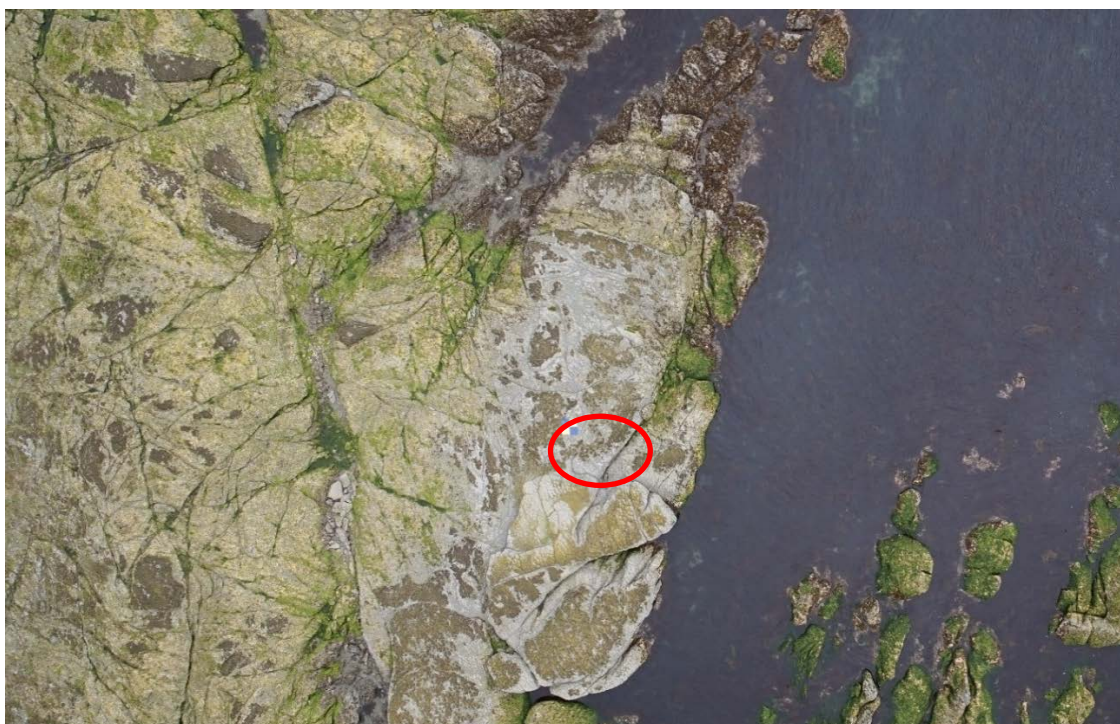
Figure 35: Example of a ground target used to geo-reference a set of UAV images.
