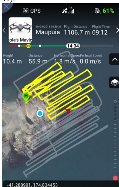
Figure 39: Image of the drone trajectories flown over Kau Bay.
