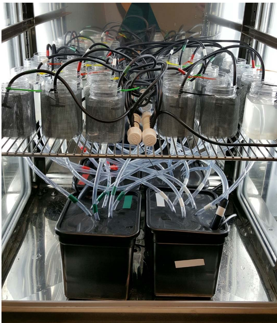
Figure A. Flow through culture set up testing temperature, shading and suspended sediment.
