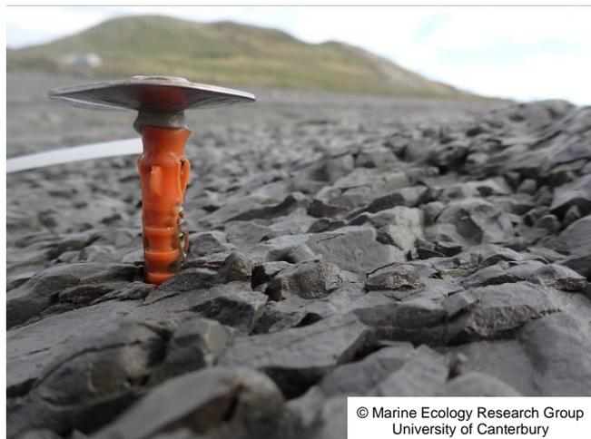
**Figure 20: Erosion rates were quantified using bolts with fixed washers by measuring the gap between the washer and the surface of the reef.**
