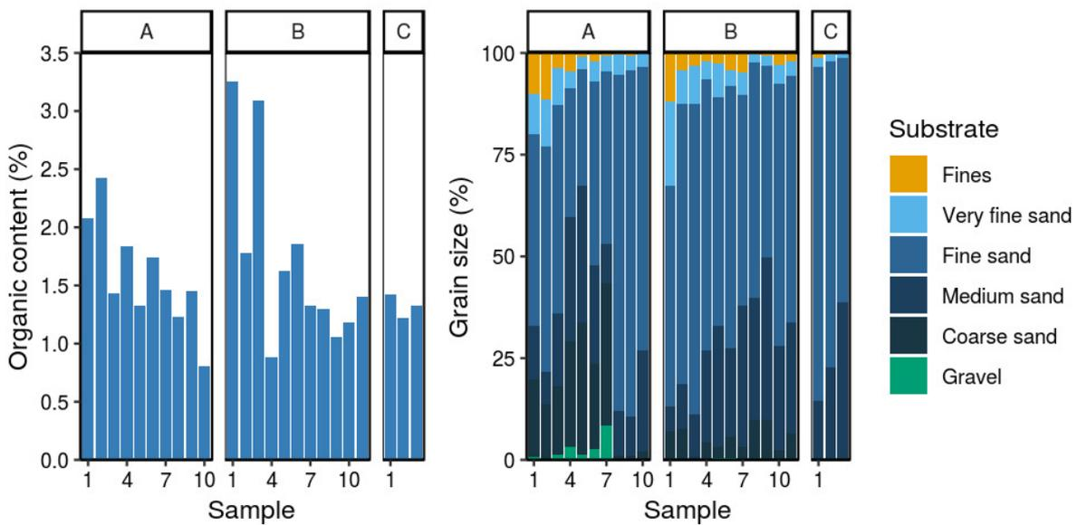
**Figure 48: Sediment sample locations and characteristics at Whangamatā Harbour. Labels correspond to stratum and sample number. Graphs show organic content (% dry weight) and cumulative grain size (%). Sediment grain size fractions include fines (silt and clay; <63 µm), sands (very fine, >63 µm; fine, >125 µm; medium, >250 µm; coarse, >500 µm), and gravel (>2000 µm) (see details in Table B-3).**
