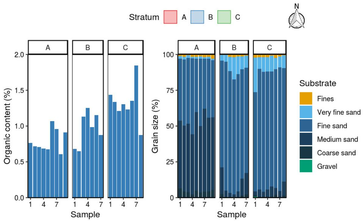
**Figure 53: Sediment sample locations and characteristics at Whangapoua Harbour. Labels correspond to stratum and sample number. Graphs show organic content (% dry weight) and cumulative grain size (%). Sediment grain size fractions include fines (silt and clay; <63 µm), sands (very fine, >63 µm; fine, >125 µm; medium, >250 µm; coarse, >500 µm), and gravel (>2000 µm) (see details in Table B-3).**
