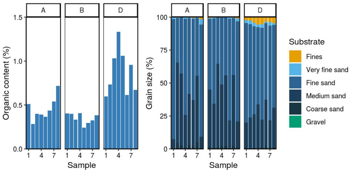
**Figure 38: Sediment sample locations and characteristics at Ruakaka Estuary. Labels correspond to stratum and sample number. Graphs show organic content (% dry weight) and cumulative grain size (%). Sediment grain size fractions include fines (silt and clay; <63  $\mu\text{m}$ ), sands (very fine, >63  $\mu\text{m}$ ; fine, >125  $\mu\text{m}$ ; medium, >250  $\mu\text{m}$ ; coarse, >500  $\mu\text{m}$ ), and gravel (>2000  $\mu\text{m}$ ) (see details in Table B-3).**
