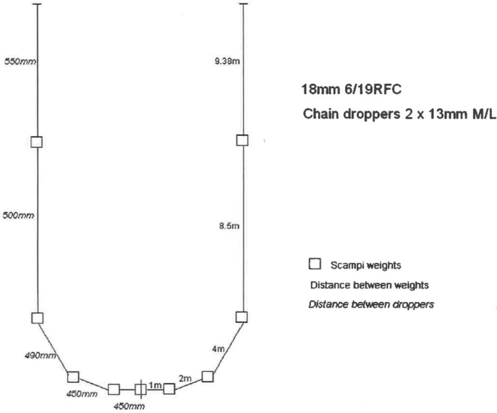
**Gear comparison between *Kaharoa* and *San Tongariro* scampi trawls (as employed during scampi surveys)**
