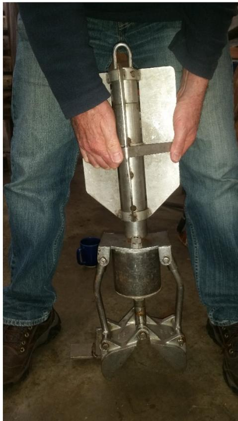
**Figure 7: Clamshell grab used to collect sediment samples during the survey.**
